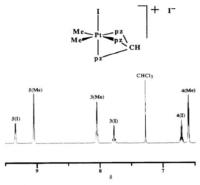
Fig. 2. <sup>1</sup>H NMR spectrum of  $[PtIMe_2\{(pz)_3CH-N, N', N''\}]I$  in CDCl<sub>3</sub> in the pyrazole ring region, illustrating the 2:1 ratio for pz environments, and resolved J(HPt) coupling for the pz group *trans* to iodine [3(I), <sup>3</sup>J(HPt) 13.2 Hz; 4(I), <sup>4</sup>J(HPt) 11.1 Hz]. *Trans* groups are shown in parentheses.
