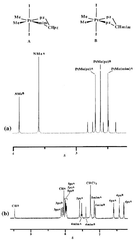
Fig. 1. <sup>1</sup>H NMR spectra of  $PtI_2Me_2\{(pz)_2(mim)CH-N, N'\}$  (2) in CDCl<sub>3</sub>, in the aliphatic (a) and aromatic (b) regions, illustrating presence of isomers A and B, and <sup>3</sup>/(HPt) for H4(mim) of isomer A (4mim<sup>A</sup>). Trans groups are indicated in parentheses in (a), and protons of uncoordinated rings are shown in *italics* in (b).
